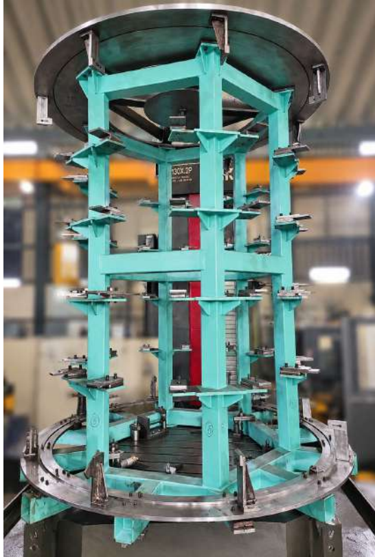
1-2M Main Assembly Fixture
