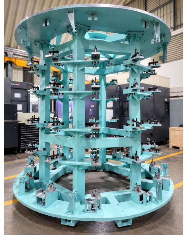
CBS Main Assembly Fixture
